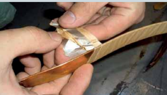
Fig. 2: Dewatering of a paper insulated conductor showing deposits of copper sulfide on the paper insulation
