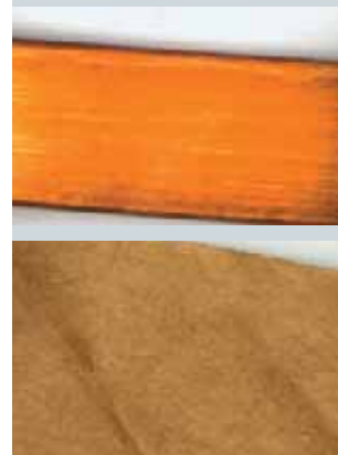
Fig. 3a: Copper and paper strips after a test with not corrosive oil
